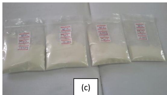
Figure 2: Photographs of the weighed starting materials of (AR) grade (a) ZnO, (b) TiO 2 and (c) MgO powders for the preparation of 80%:20%, 60%:40%, 40%:60% and 20%:80% ZnO:MgTiO 3 composite materials
